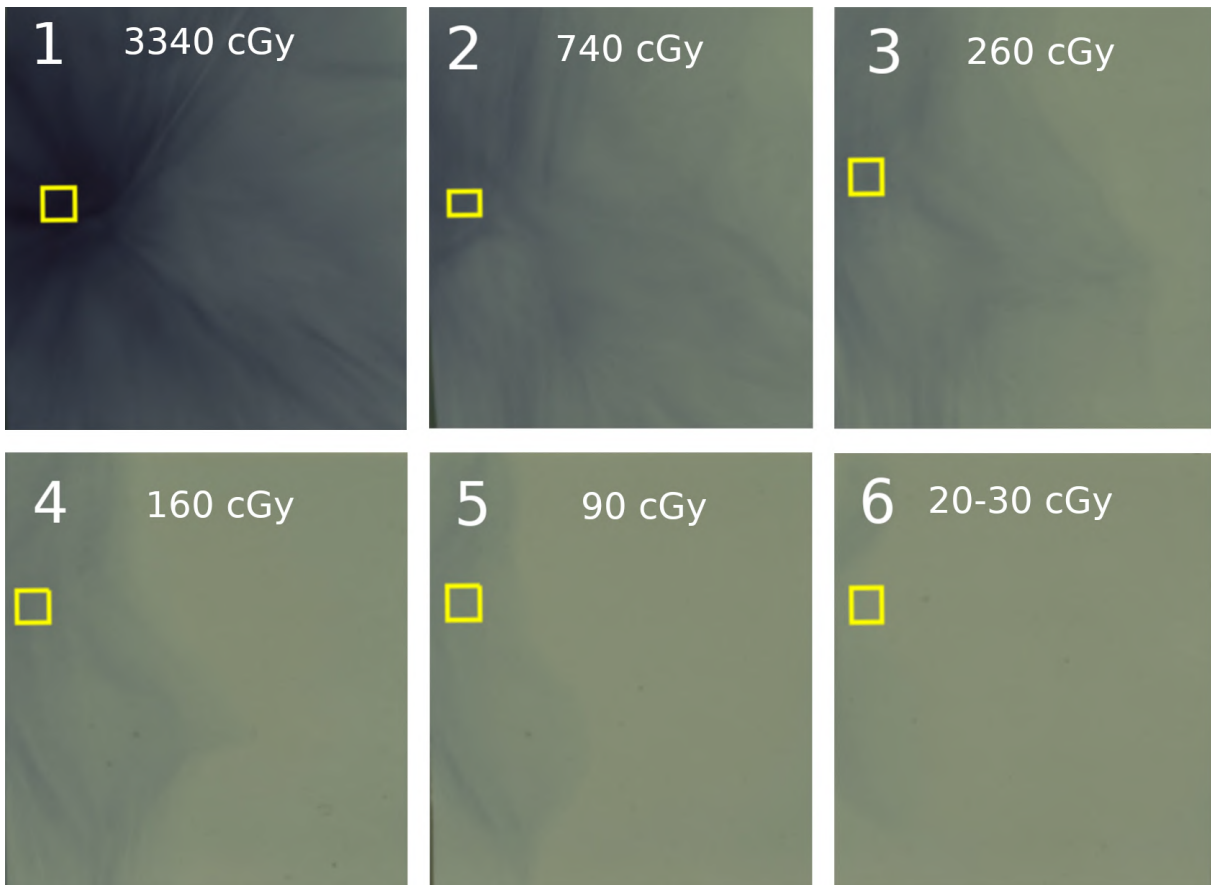
Figure 3.9: Example of EBT stack irradiated with one shot during the ELIMAIA commissioning experiment. Layer 1 is at the front and layer 6 at the back. The films are also annotated with the absorbed dose in cGy. A 45\ \mu\text{m} Al filter was placed in front of the stack to block heavy ions and low energy protons.
