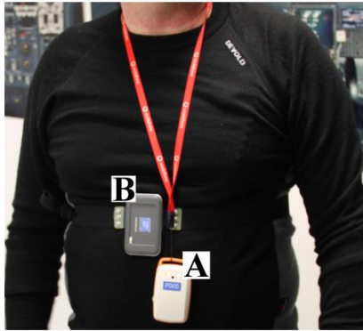
Fig.1 Measuring system with modular sensing unit (A) and a respiratory rate sensor (B).
