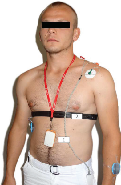
Figure 2. Measuring system with modular sensing unit (1) and a heart rate sensor (2)
