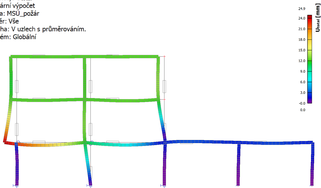
Fig. A-33. Maximal linear elastic deflections of adjusted model at extraordinary ULS in [mm].
