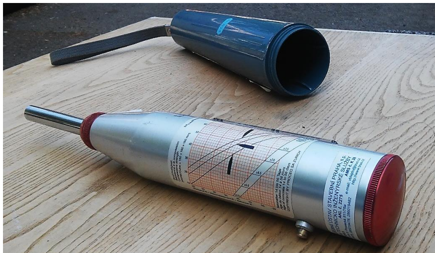
Fig. 6-3. Classic Schmidt rebound hammer, Proceq model N.
