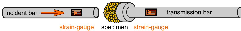
Fig. 3. Principle of the direct impact Hopkinson bar method.
