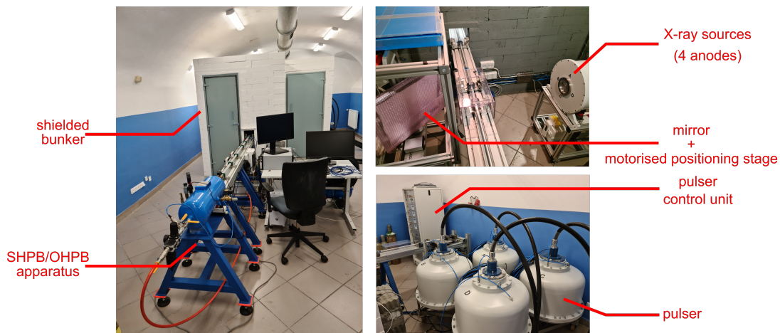
Figure 3.3: Experimental facility for the high-speed X-ray imaging during the high-strain rate testing.
