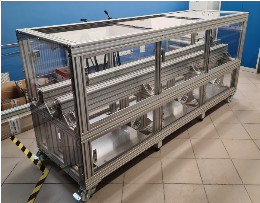
Figure 3.4: Frame of the assembled loading device
