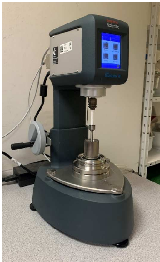
Obr. 4.19: Reometr Thermo Scientific HAAKE Viscotester iQ
