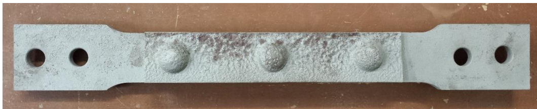
Fig. 37 Photo of tested specimen with a medium level of corrosion (Example of a sample from group 2)
