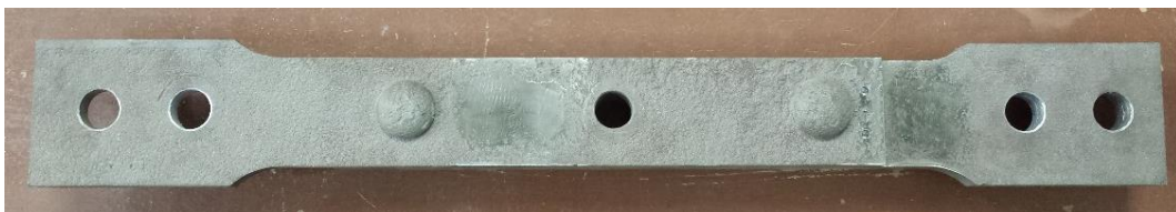
Fig. 39 Photo of tested specimen with a missing rivet (Example of a sample from group 4)
