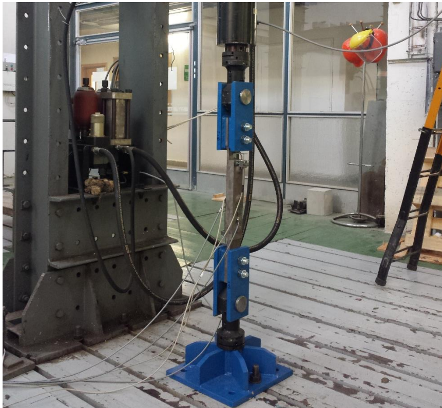
Fig. 59 Arrangement of the fatigue test; the specimen fixed by the fixing device
