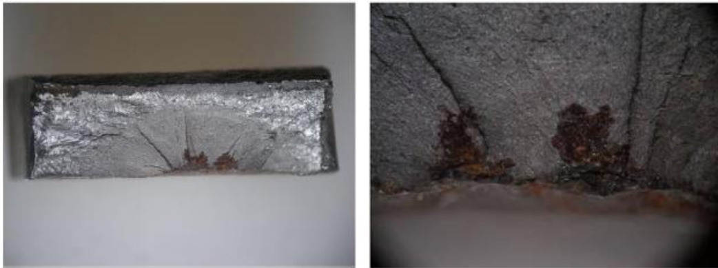
Fig. 11 Fatigue damage of the tested specimen [25]
