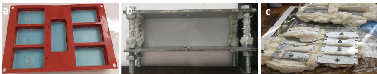
Figure 18: Sandwich preparation : a) Mold used to prepared rectangular plates, b) Form used to prepare the PE/PU sandwiches, c) Samples foaming.
