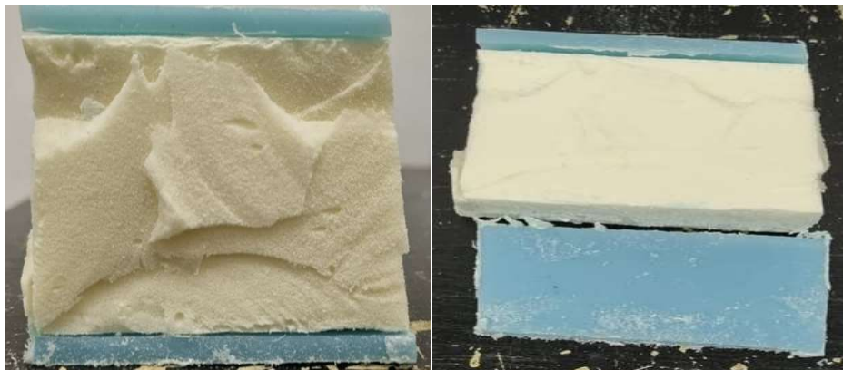
Figure 89: Sandwich prepared using untreated powder before testing.
