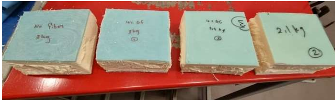
Figure 23: Specimens for falling weight testing before the test.
