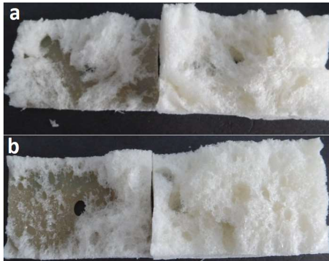
Figure 53: PU residue: a) Plates prepared from 3 min treated powder, b) Plates prepared from 5 min treated powder.
