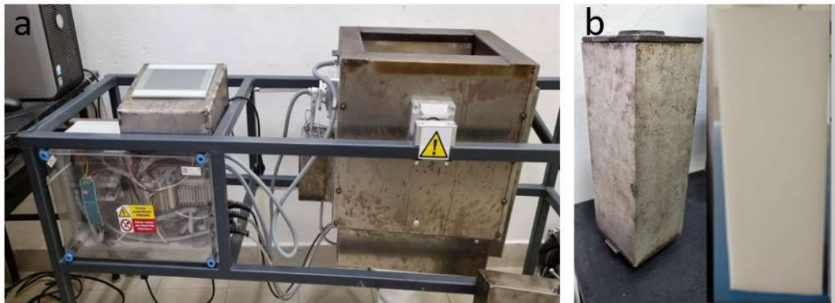
Figure 17: a) "Rock-and-roll" Rotational molding machine, b) Aluminum mold .
