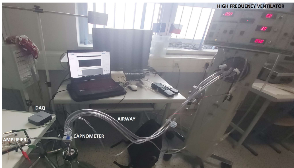
Figure 5.12: Laboratory setup for high frequency ventilation testing
