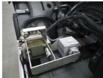
Hytrans® truck hydraulics kit. For connecting the HRU.
