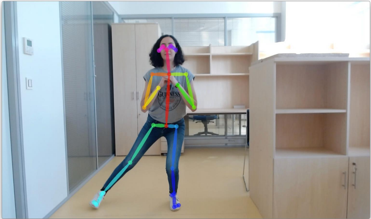
Figure 8: Video with OpenPose skeleton for each frame
