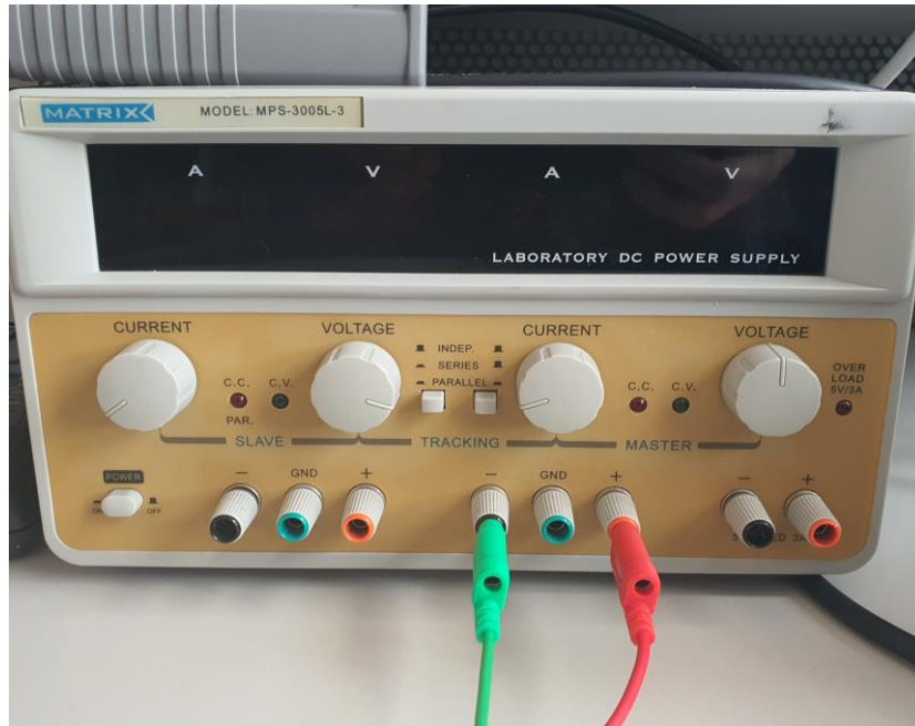
Figure 7.1 Connection of power supply to pressure transducer
