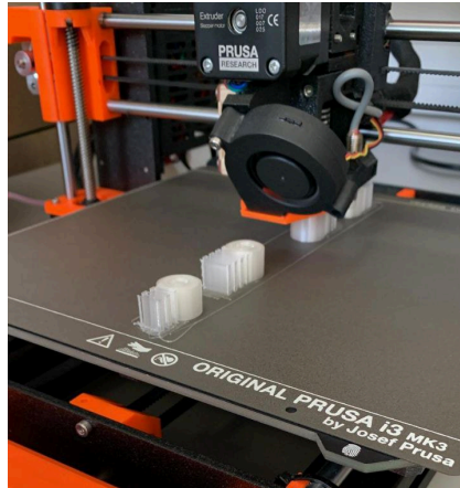
Figure 4.18: 3D printing process of Version 1 designs.
