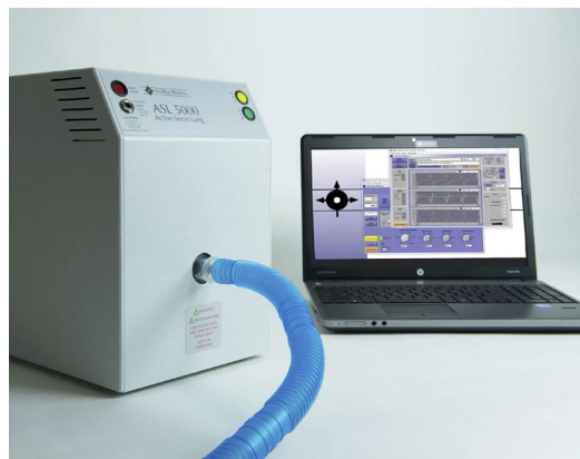
Figure 2.7: ASL 5000 lung simulator taken from [24]
