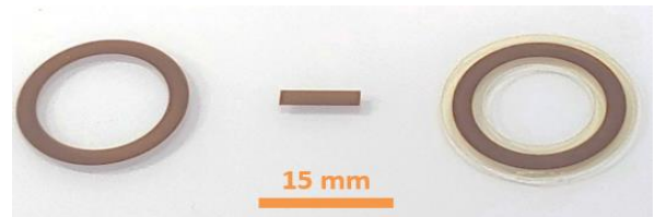
Fig. 5. Ring-shaped inkjet-printed core (left) and inkjet printed UV cured coating (right). The straight bar (middle) is a sample printed for SQUID measurements.
