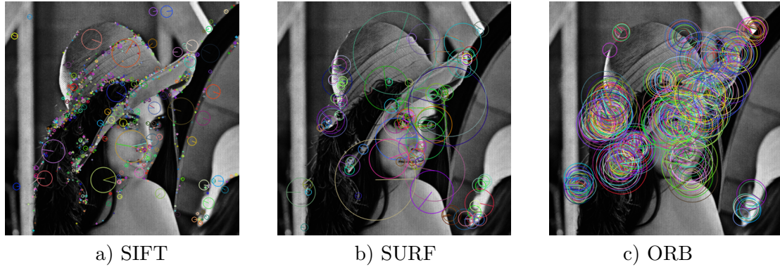
Figure 4.2. Comparison of SIFT, SURF and ORB interest points. Circles denote the scale of the interest point and the inscribed line the direction of the feature.
