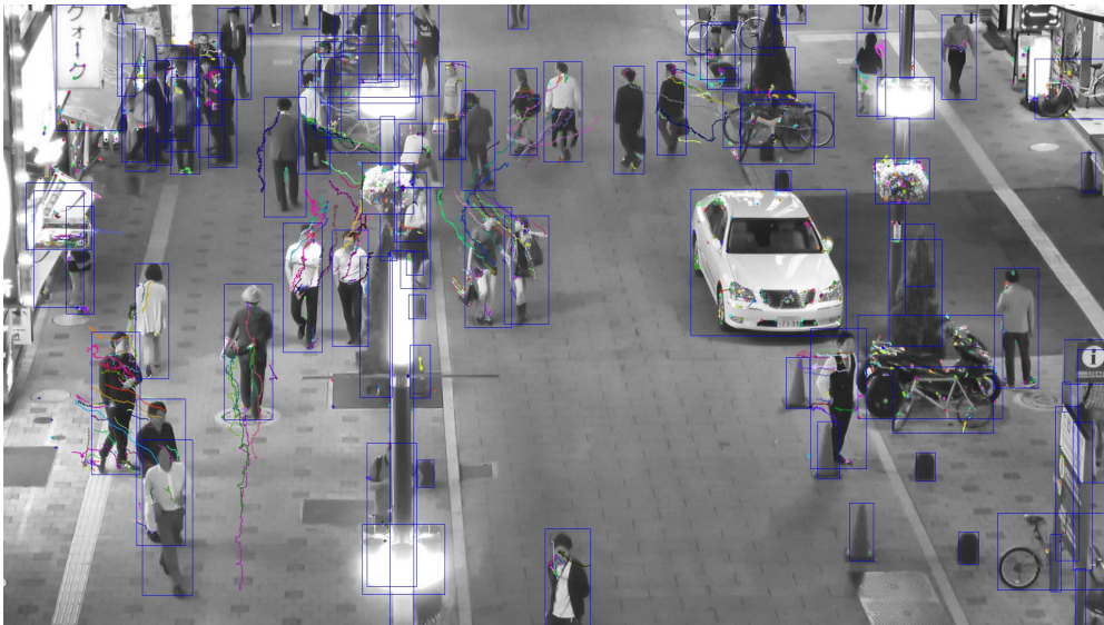
Figure 7.4. Resulting tracklets from sequence MOT17-04, valid in the displayed frame (some are already lost). Ground truth bounding boxes are shown in blue.
