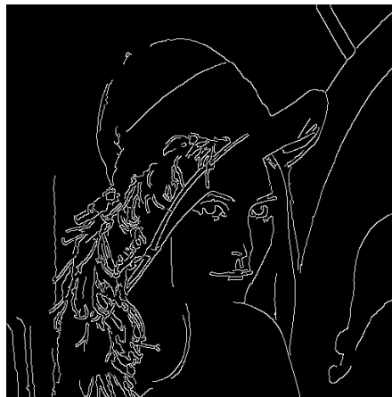
Figure 4.1. Result of Canny edge detector, 1\sigma Gaussian blur and 10 – 30% threshold.
