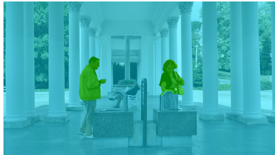
Figure 7.6. Result of frame segmentation based on clustering of estimated motion vectors according to their angle and size and providing the clustered visual features as inlets of the Grid Cut algorithm.
