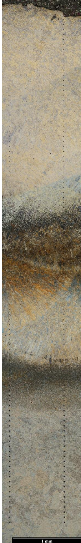
Figure 56: Image of a cross-section of the clad with visible microstructure and indents.
