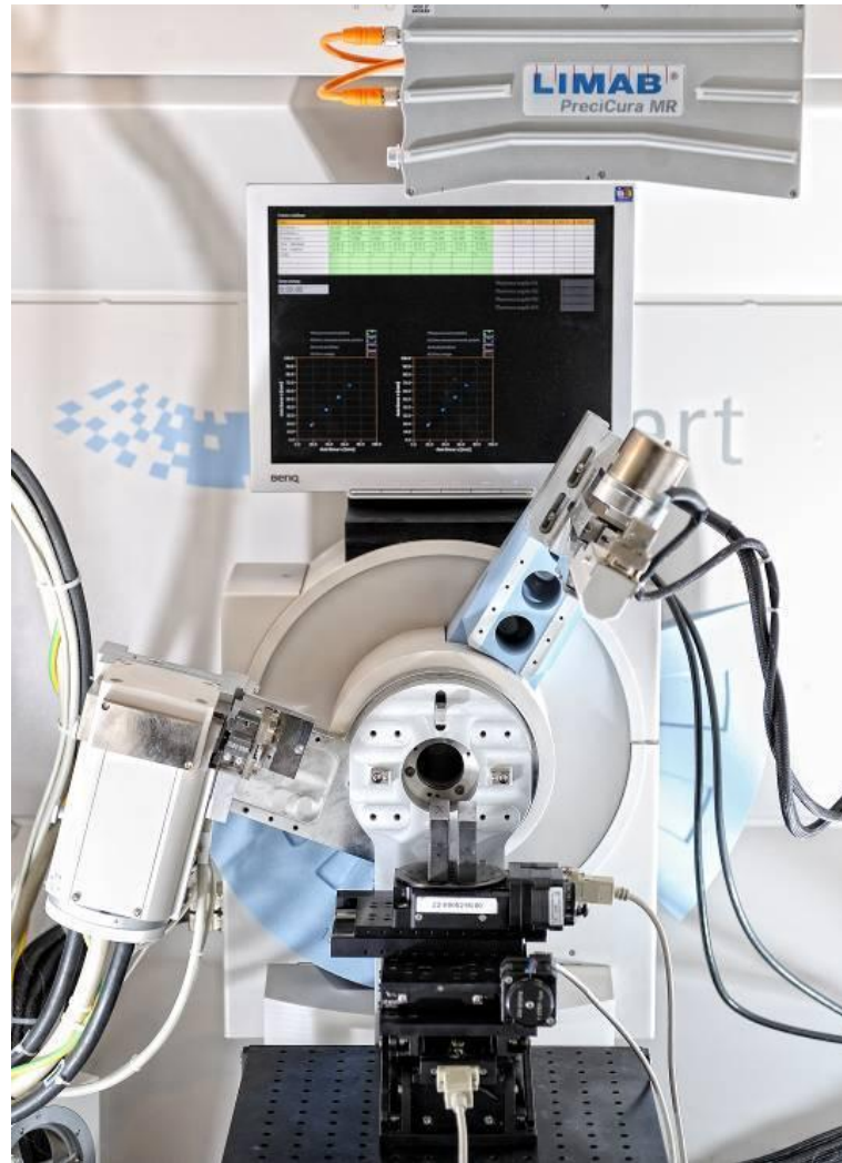
Figure 24: X'Pert PRO MPD diffractometer with four-axis positioning device and triangulation laser.
