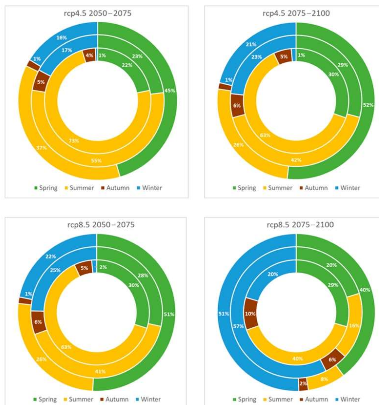
Figure 7. Example of the number of peak months over the return period 1 in 20 years per scenario—rivers within Elbe basin; catchment size: inner circle—451 km 2 , middle circle—1157 km 2 , outer circle—41,831 km 2 .
