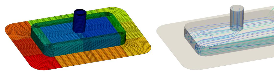
Decomposed computational mesh (left) and streamtraces with coloring by the magnitude of velocity (right)
