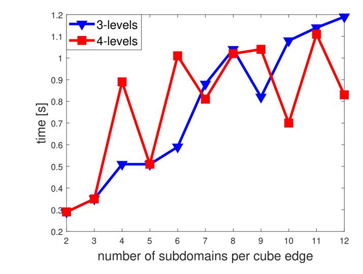
Comparision of 3- and 4-level method. Mean time for setup, mean time for the BiCGstab iterations and mean total time (left), mean time for one iteration (right).
