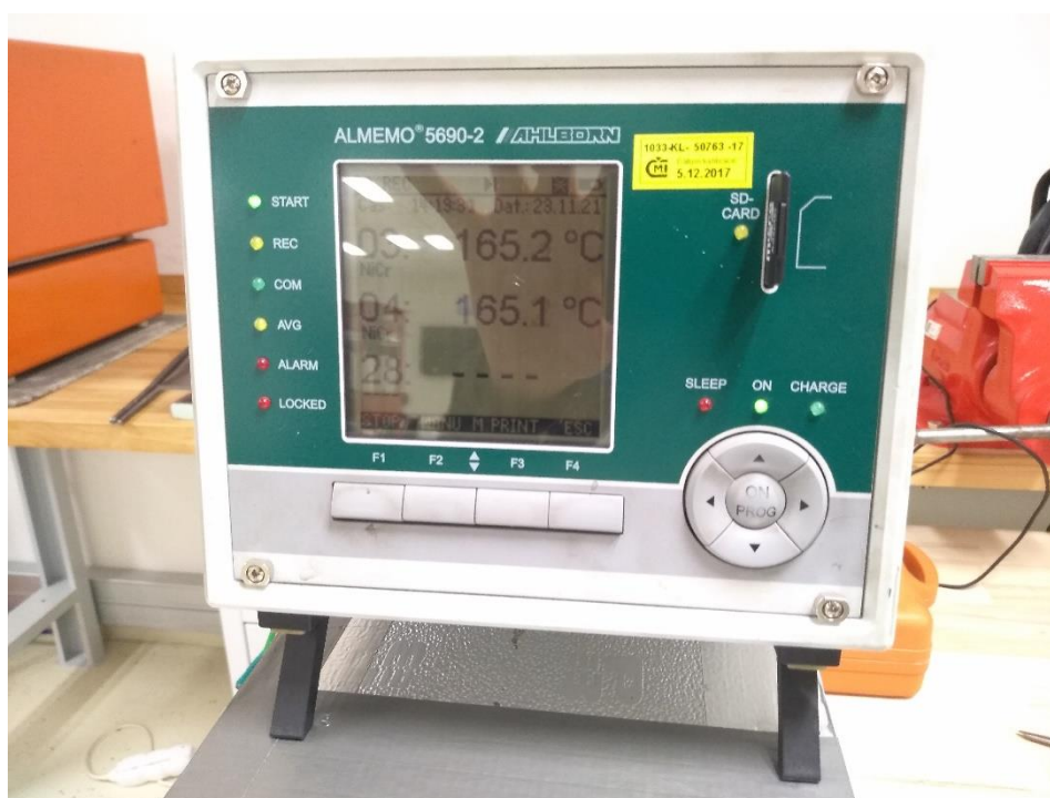
Obr. 50 - Datalogger AHLBORN ALMEMO 5690-2
