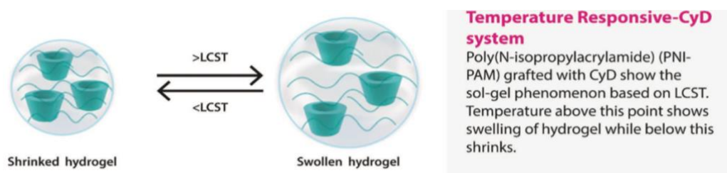
Figure 2 CD-based Hydro/Nanogel Swelling showing characteristic changes above and below LCST/VPTT critical temperatures for a CD-co-NIPAM hydrogel ( 32 ). The blue cone structures are representative of the included CD cone like cavity structures responsible for hydrophobic drug encapsulation in the nanogel complex.
