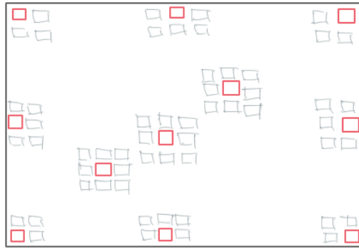
Figure 8.18: Check neighbourhood method, forming neighbourhood, depending on the position of the checked cell
