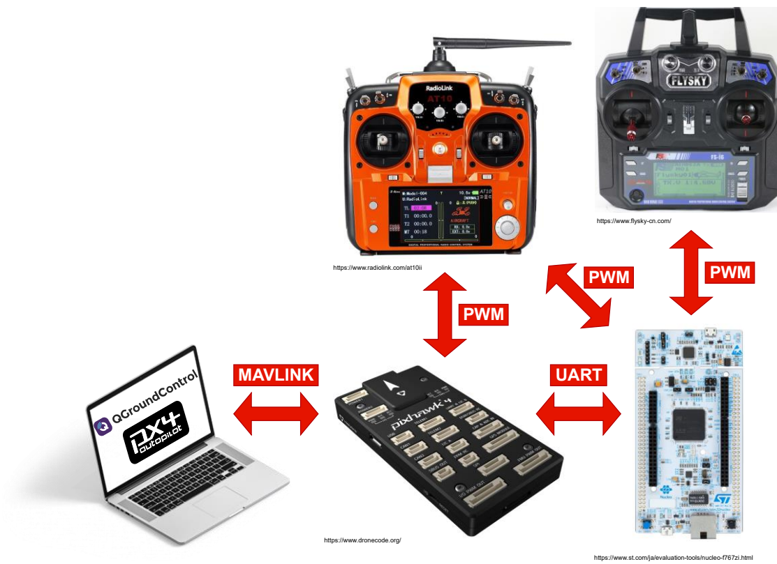
Figure 33 Device communication overview
