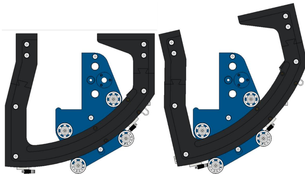
Fig. 38: Rib assembly in minimum and maximum tilt position
