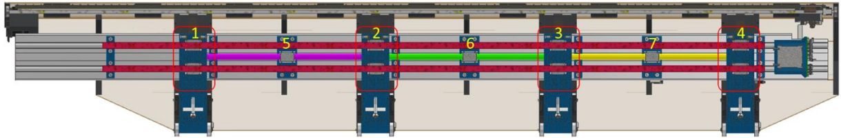
Fig. 34: Guide rods system for the carriage
