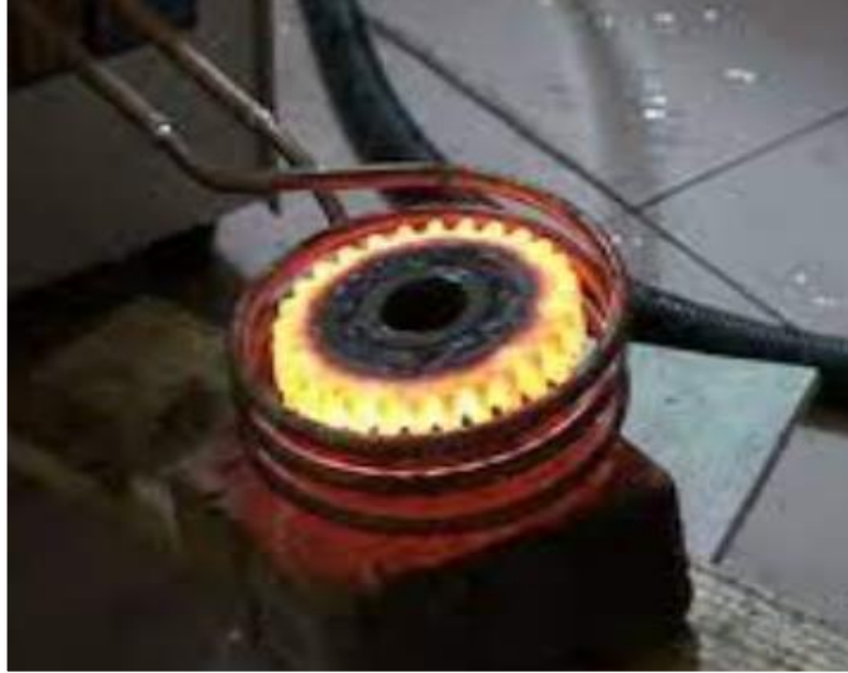
Figure 7 Gear quenching by Induction heating coil
