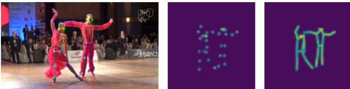
Figure 4.3. Heatmap visualization. Picture with a skeleton pair on the left, keypoints heatmap in the middle and limbs heatmap on the right.
