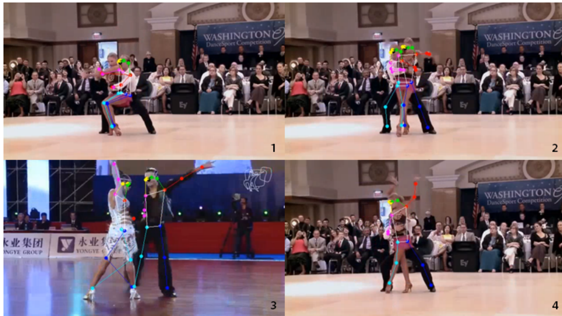
Figure 5.5. HRNet pose estimation errors. 1) Doubled skeleton into a single person 2) Switched body parts 3) Wrong keypoint connections 4) One skeleton out of two people
