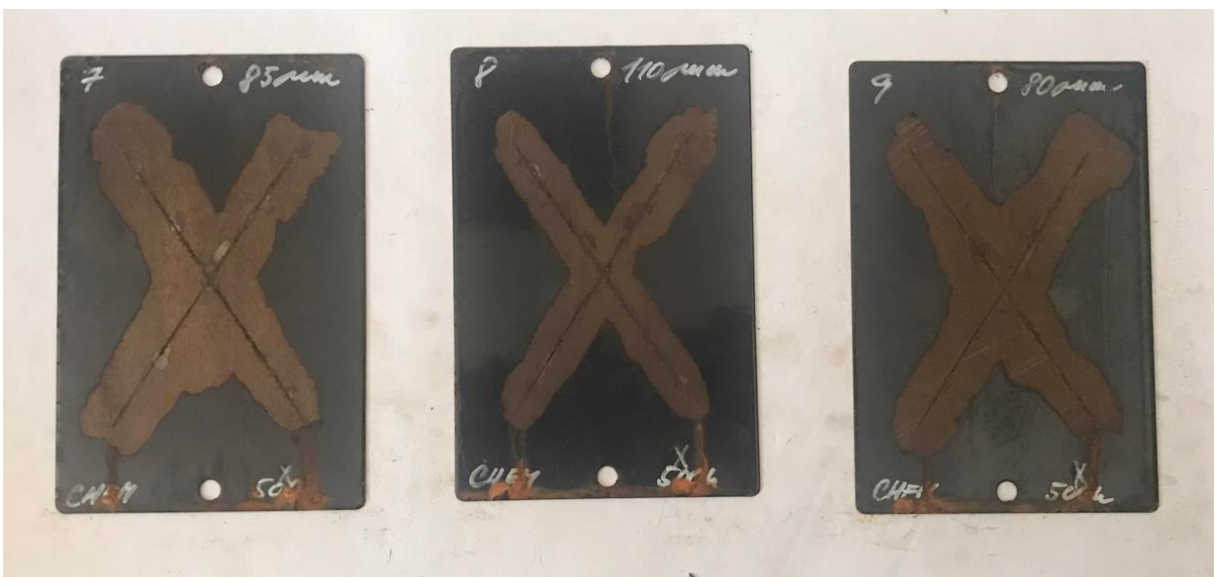
Obr. 40 - Chemetal: HRS, 3x 500 h
