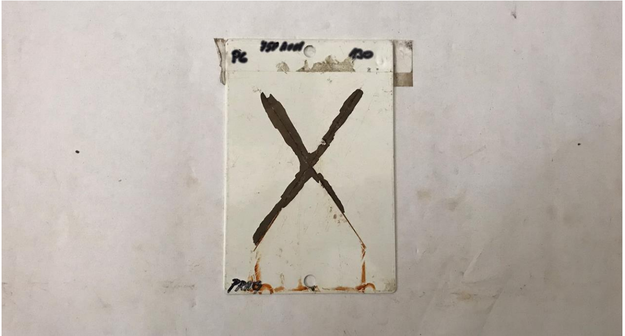
Obr. 27 - Pragochema: RAD 10 + Fos 2061, CRS: 750 h
