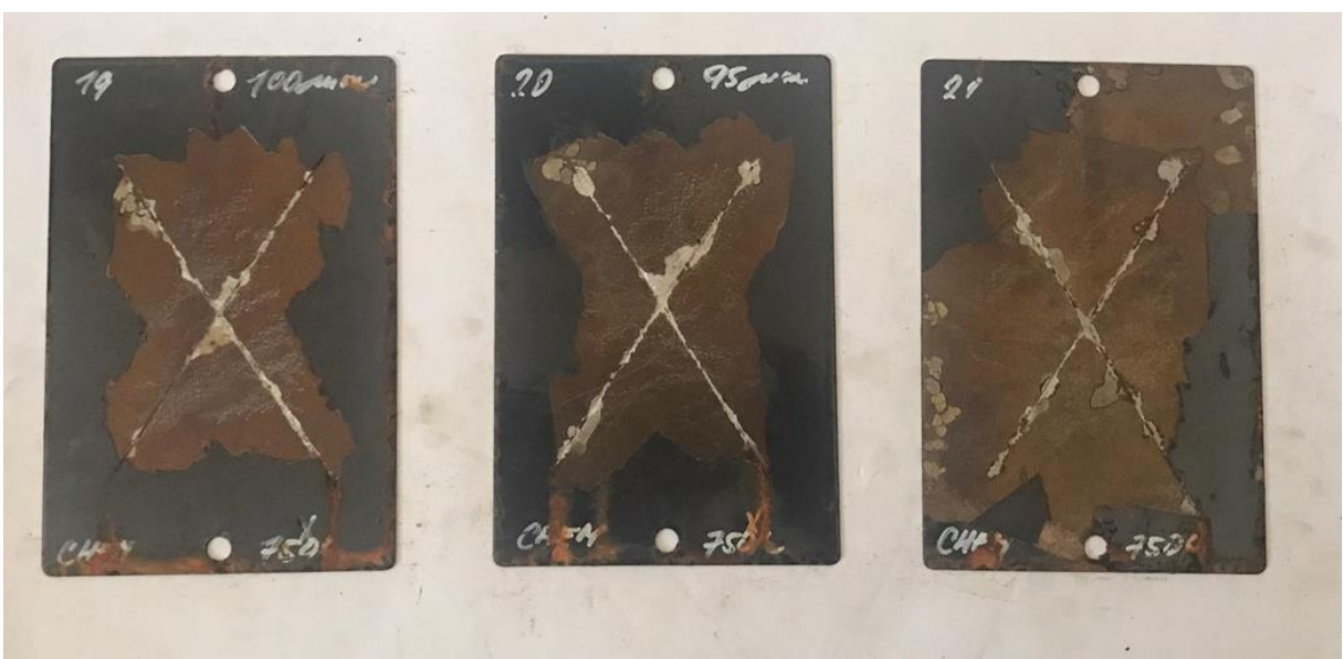
Obr. 44 - Chemetal: HRS, 3x 750 h
