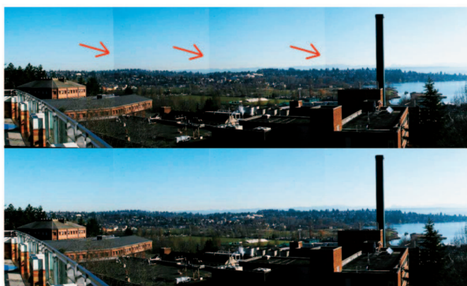
Figure 4.2.1: Stitched image exhibiting vignetting. Image courtesy of [35].
