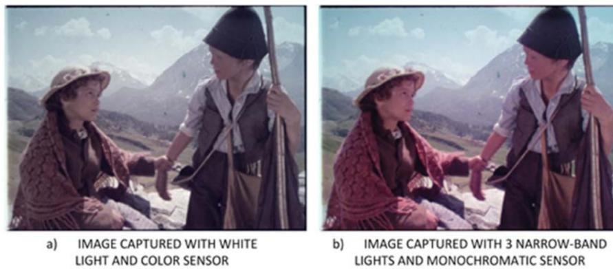
Figure 2.3.3: Comparison of film scanned with white/composite lights and color/monochrome sensors. Image taken from [25].
