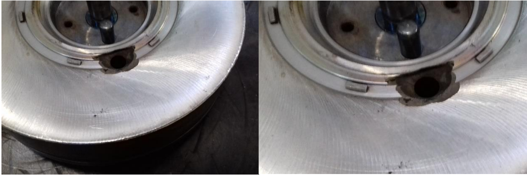
Figure 29 : Breakdown due to forcing when closing the machine
