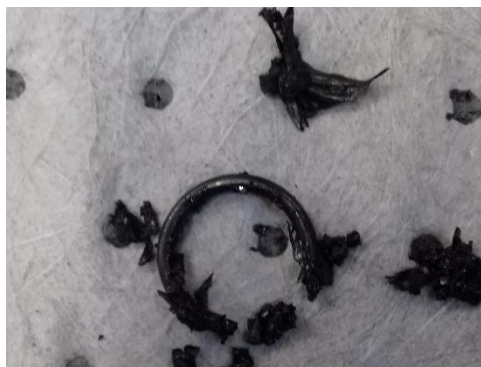
Figure 23 : Damaged O-ring found after leakage
