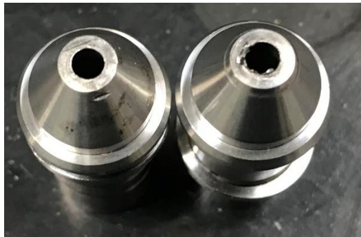
Figure 30 : Damage on the nozzle due to the needle forcing
