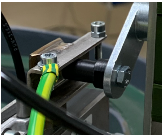
Figure 2.5: Crank and slit - vertical scraper
