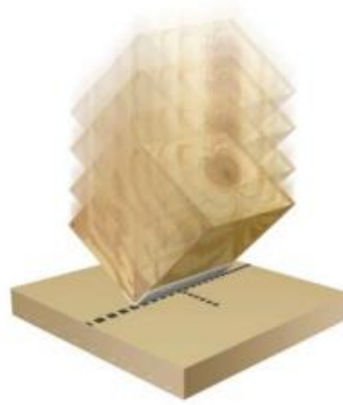
Obr. 9: Concentrated Impact Test Procedures dle ISTA 6-FedEx-A (převzato z [14])
