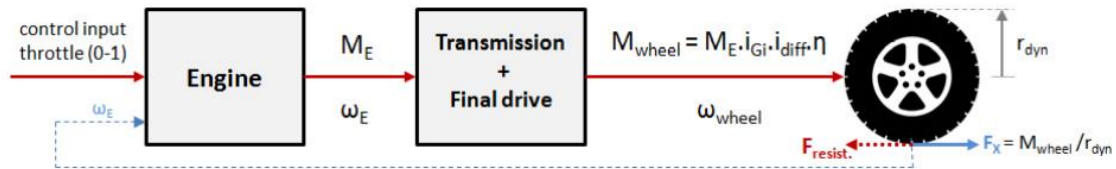
Figure 23 - schematic powertrain Simulink model [20]
