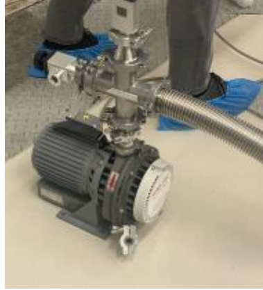
Figure 53: Vacuum pump connected to pressure sensor through valve top flange
