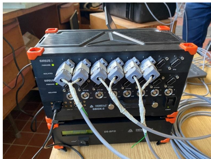
Figure 48: Six DB9 connectors connected to DAQ to complete compensation circle of the three strain gauges
