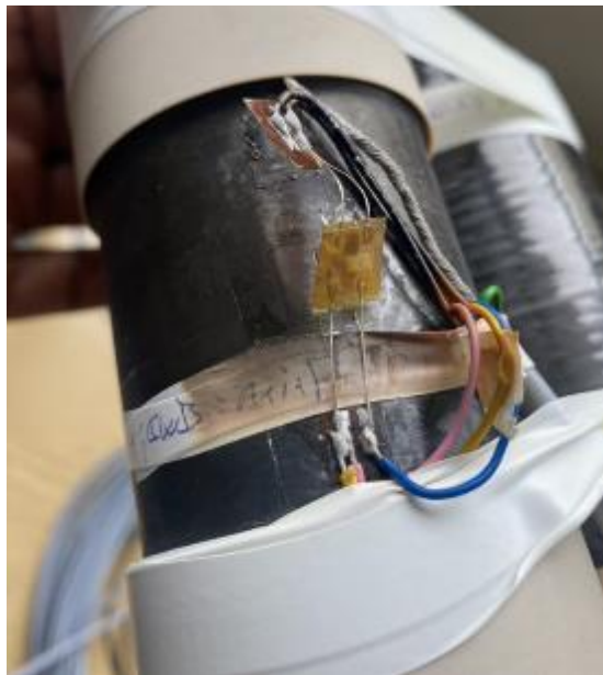
Figure 63: Irradiated Sample pipe (No.2), peeled off strain gauge
