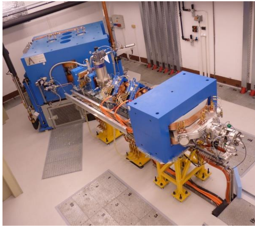
Figure 50: Cyclotron TR-24 of the canadian company ACSI (Advanced cyclotron systems Inc.) in the Czech academy of sciences irradiation chamber.
