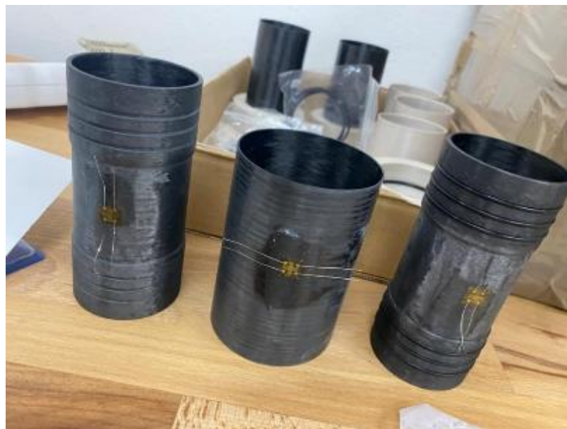
Figure 45: Applied Strain gauges on pipes
