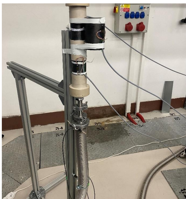
Figure 58: Pipes sample assembly taped to metallic framing and connected turbomolecular pump hose.
