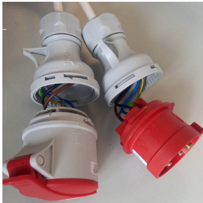
Figure 4.13: Input (right side) and output (left side) MPD cables
