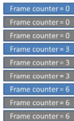
Figure 5.16: Frame Counter in VoSPI protocol [32]
