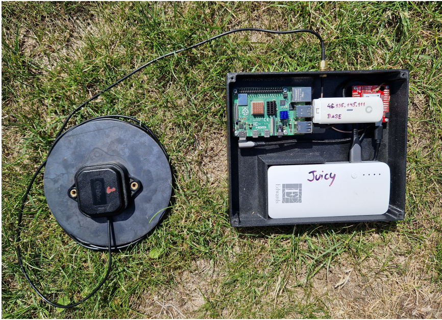
Figure 6.3: A picture of final Base Station printed out and planted with Raspberry Pi, U-Blox ZED F9P, USB internet modem and power bank. On the left finds itself a multi-band antenna with a steel disk similar to the one used at the ToMi2 platform.
