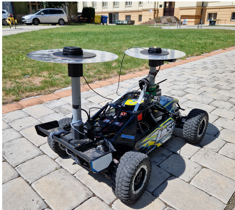
Figure 6.4: 3D printed models holding dual antenna setup on the ToMi2 vehicle.
