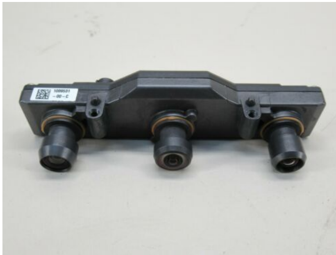
(b) : The Tesla triple front-facing camera setup, placed above the rear mirror. The cameras on the sides combine to form a calibrated stereo pair to create a 3D depth representation of the space in front of the vehicle. The central camera with magnifying optics serves for long-range detection purposes. [70]
