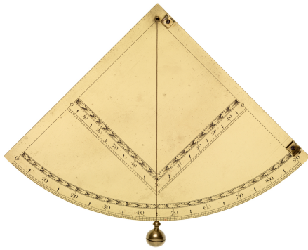
(a) : A quadrant, firstly invented for astronomical purposes, was later used to measure angles of the Sun and stars in the night sky, allowing sailors to navigate more accurately based on the knowledge of star constellations' position. [17]
