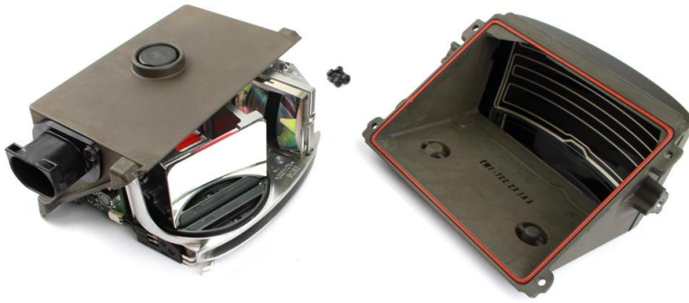
Figure 3.13: A commercial Valeo Scala 2 LiDaR with a rotating mirror used for beam steering. [68]
