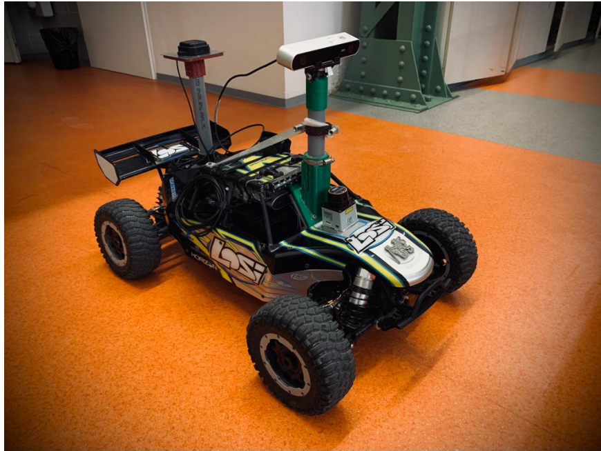
Figure 5.1: Toyota Mini 2 RC overactuated platform, with an old Sterolabs Zed 1 camera and a single band GNSS receiver.
