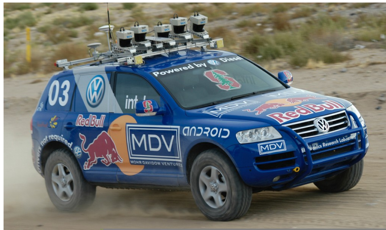
Figure A.5: The 2005 winning car, Stanley, based on the VW Tuareg platform. The vehicle was equipped with a series of LiDARs on the roof, GNSS suite, accelerometers, odometers and a front-facing camera for localization and drive-by-wire executed Stanley control law for driving. [23]
