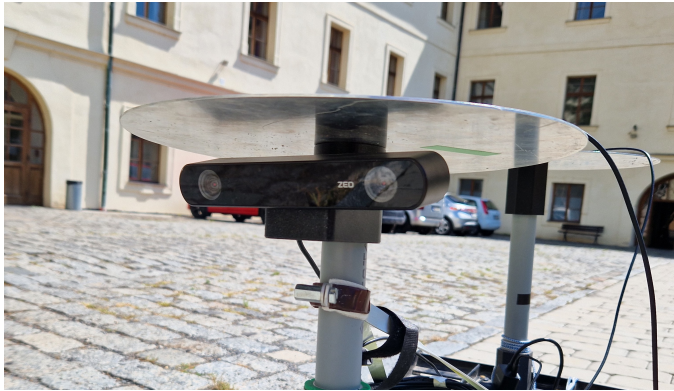
Figure 5.3: StereoLabs Zed2 stereo-camera bolted to a new mount for camera and DGNS antenna, which I have created(paragraph 6.2).
