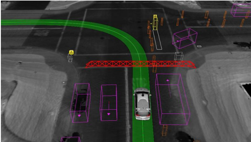
Figure 1.4: Waymo's local localization and planning for their autonomous vehicle. We can see that the car distinguishes different types of obstacles and correctly plans its course to avoid a collision. [8]
