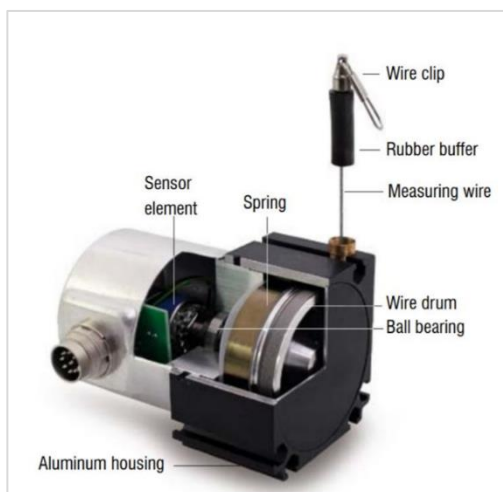
Figure 12: Draw-wire sensor [ME19]
