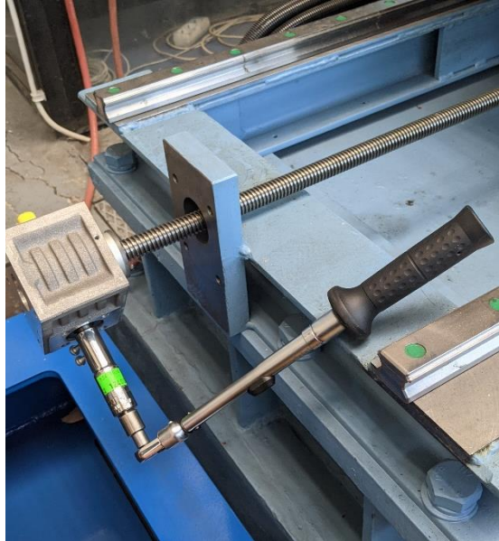
Figure 23: Torque measurement using wrench
