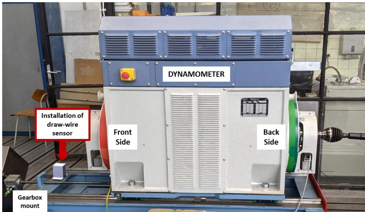
Figure 61: Draw-wire mounting location recommendation
