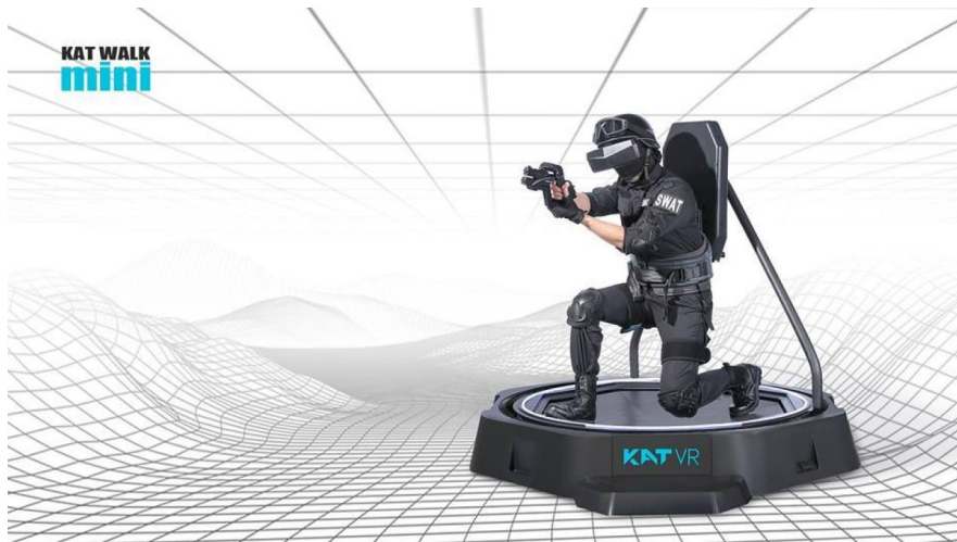
Figure 2.11: Example of a non-physical VR locomotion controller[10]
