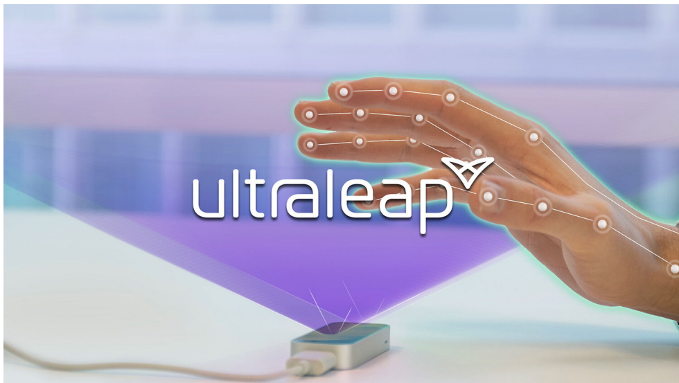
Figure 2.9: Example of an optical hand motion tracker[9]
