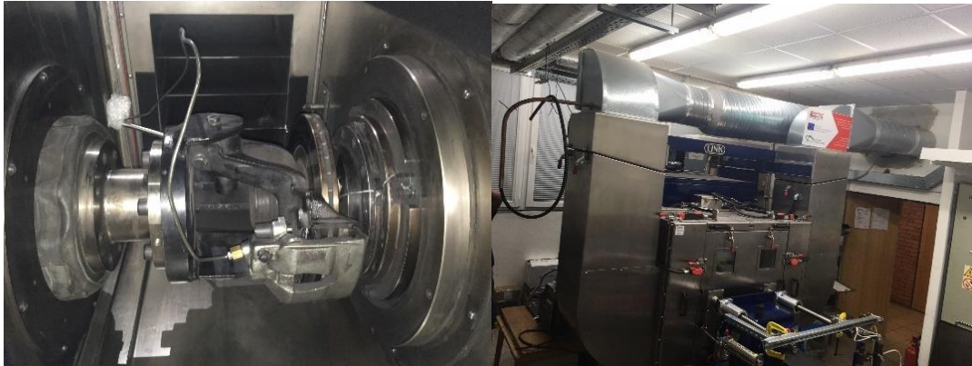
Figure 10. Experimental Setup of the brake disc on the dynamometer
