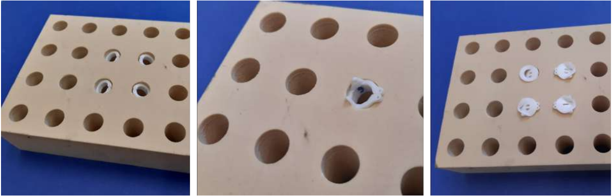
Figure 61: Specimens after asymmetric push-in test performed on polymeric burr hole rings and corresponding polymeric burr hole cups.
