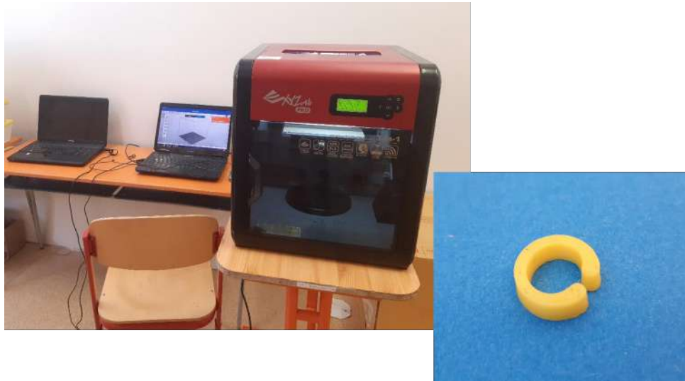
Figure 29: Manufacturing of pre-prototype burr hole ring.
