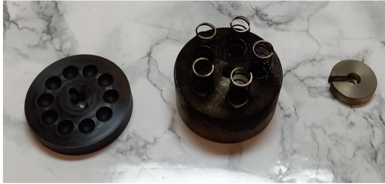
Figure 55: Clogged and possibly damaged parts of the RDD
