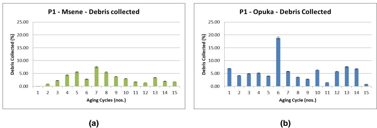
Graph 8: Average Debris brushed off from (a) Mšené stone (b) Opuka stone aged with procedure P1
