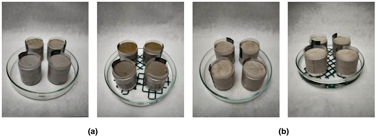
Figure 11: Example of RILEM samples partial immersion before and after salt contamination (a) Mšené (b) Opuka
