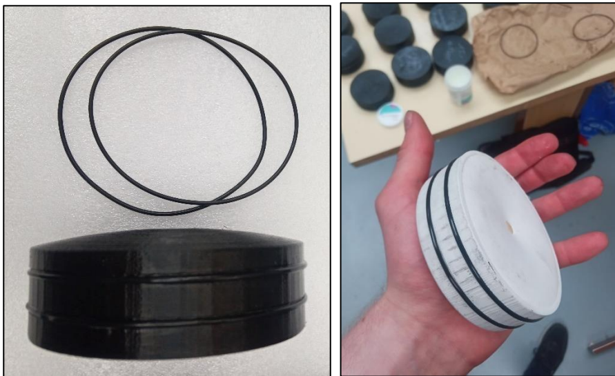
Figure 20: O-rings (size inner \varnothing 95 mm, thickness 2mm) and petroleum jelly are applied.
