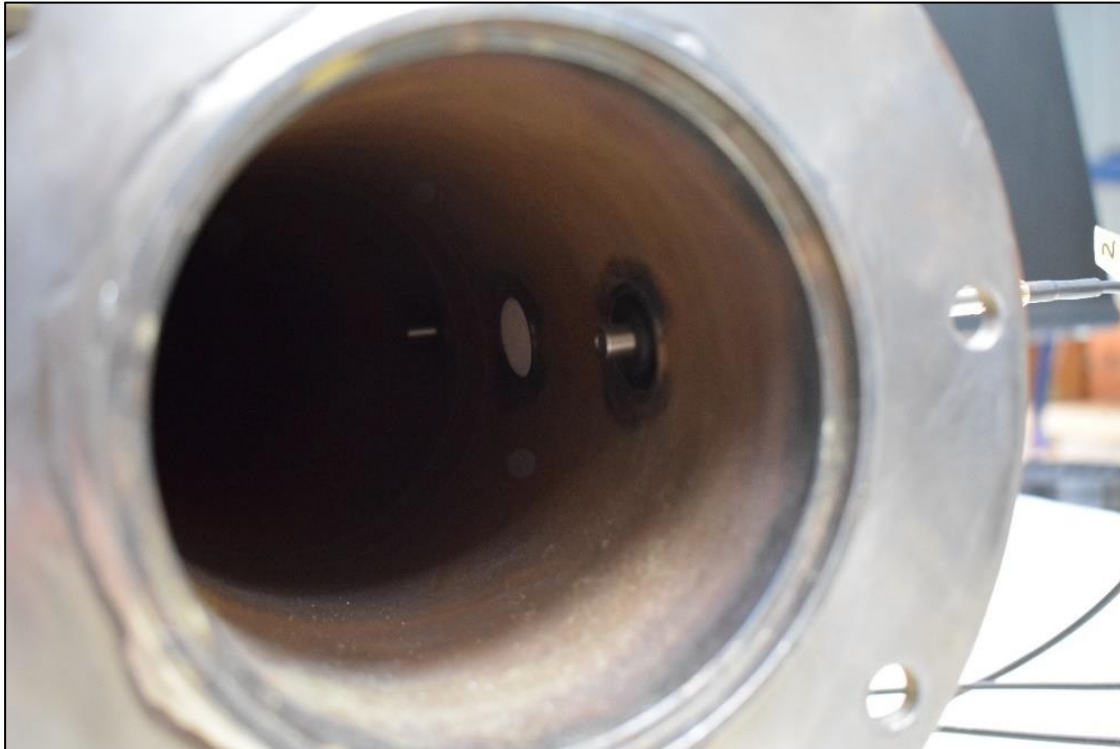
Figure 23: Microphone stick out seen from the inside of the tube (note here the microphones are sticking out too far .)
