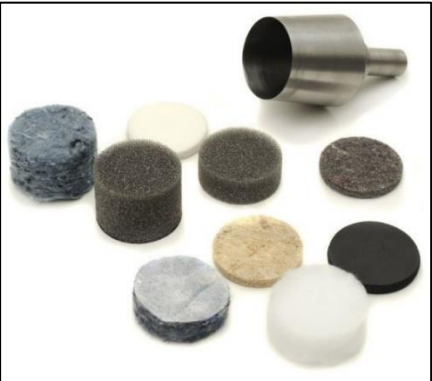
Figure 11: Typical acoustic test samples, with a sample cutter. [19]
