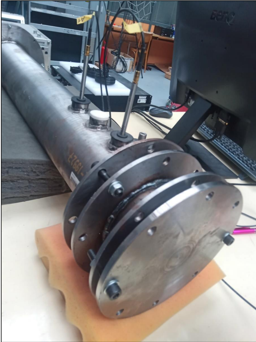
Figure 26: Used two microphone setup in the lab, The sample is always placed in the same place and backed by a 20 mm thick steel plate.
