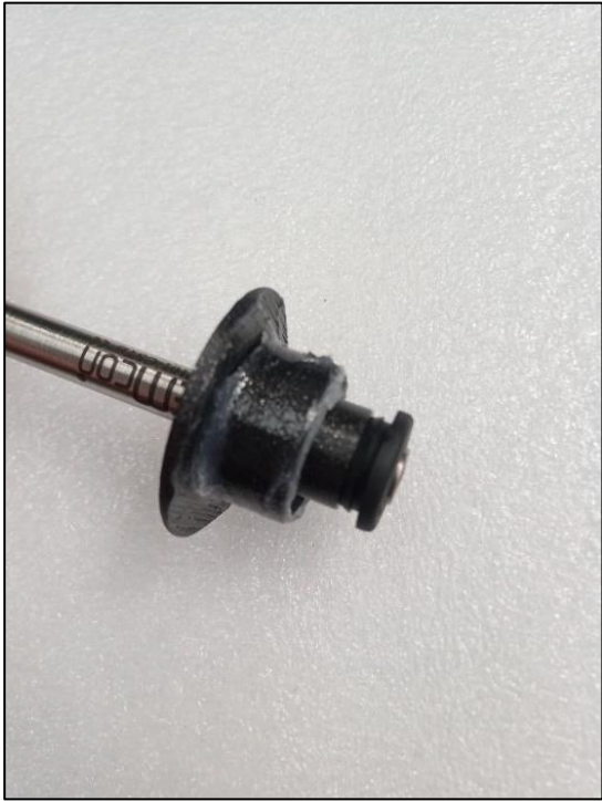
Figure 17: Microphone mounted in plastic holder that is installed in the tube using a friction fit and petroleum jelly. The microphone stick out is measured here.
