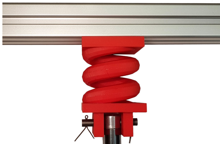
Figure 6.6: The detail of the damping spring made of PLA
