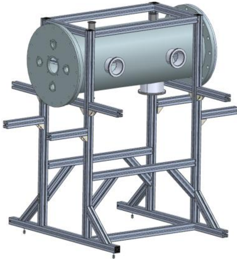
Figure 29 – The supporting construction of the vacuum chamber [26].
