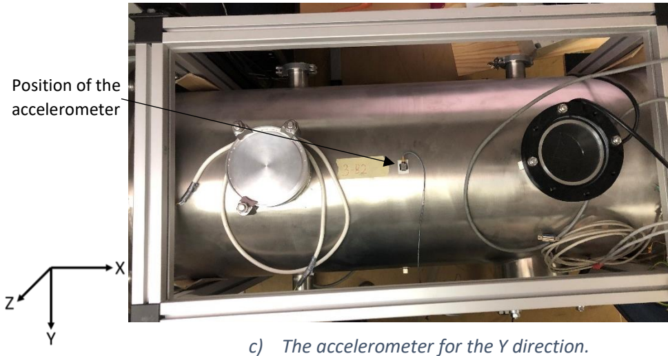
Figure 8 – The setup of the experiment to measure the noise of the environment.
