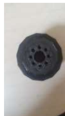
Figure 25: Joint face, notice the polygon shape instead of round.
