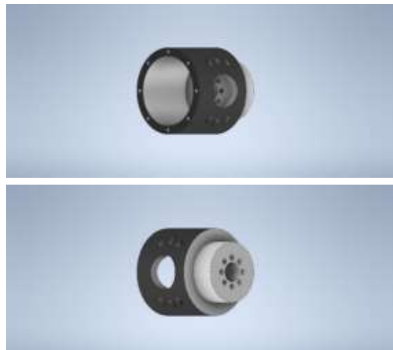
Figure 19: First joint segment, 2 views
