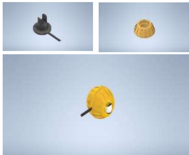
Figure 21: Parts of ball wheel and final assembly
