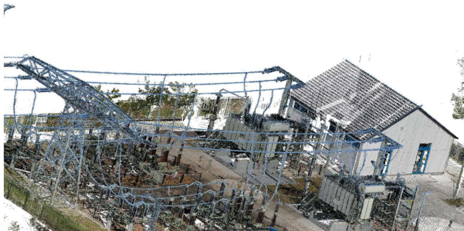
Obr. 11: Model rozvodny, RIEGL LMS Z360 [Geodis, 2004]
