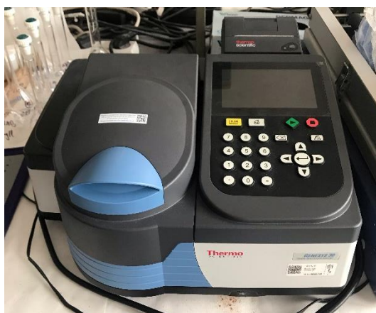
Fig. 6: Spectrophotometer Thermo Scientific GENESYS 30 Vis
