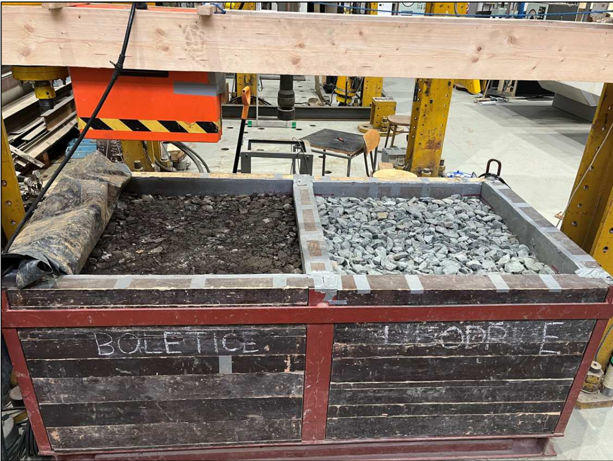
Obr. 33: Model M5-8 a M5-4: Vlevo kamenivo Boletice nad Labem, vpravo kamenivo Libodřice
