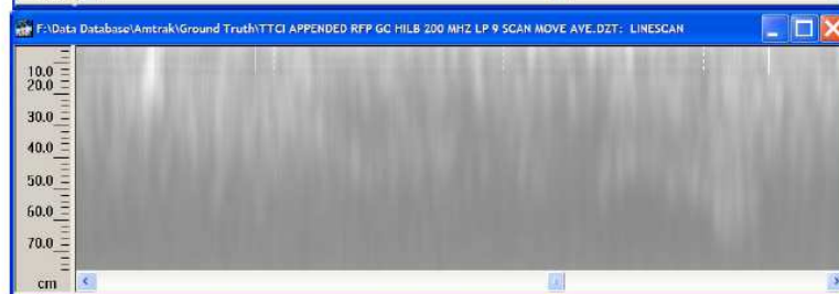
(b) Processed GPR Data: Scattering amplitude envelopes
