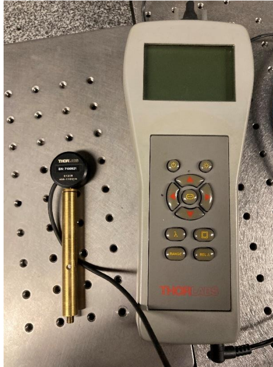
Figure 5.15 Optical power meter THORLABS
