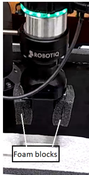
Figure 4.14: Actual test of parallel gripper with foam blocks attached to the fingers at HennLich s.r.o. using Hanwha cobot.[36, 11]
