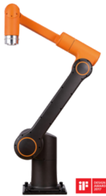
Figure 3.24: A 6-axis Cobot from Hanwha manufacturer.[11]
