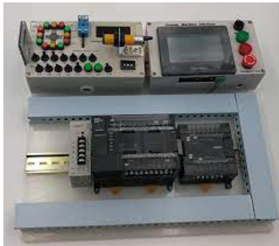
Figure 6.16: PLC and HMI from Omron manufacturer.[27]
