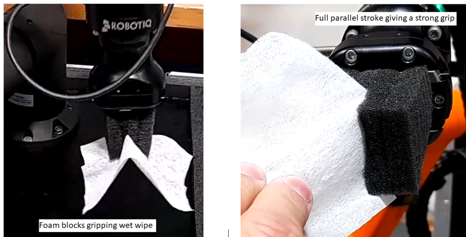
Figure 4.15: Testing of gripping of wet wipe and strength of grip using foam blocks.[36, 11]
