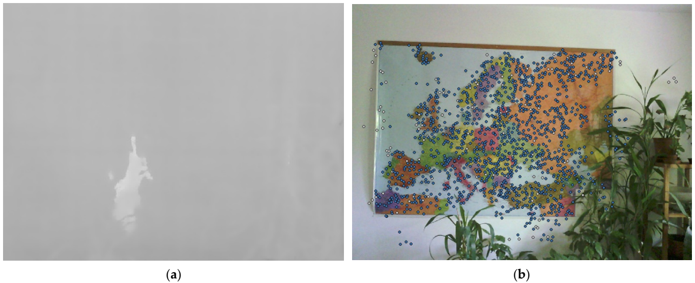
Figure 2. TIR and RGB image of the same scene: (a) Feature matching algorithm failed to find any key points or tie points; (b) Feature matching algorithm found a sufficient number of tie points (blue dots) [28].
