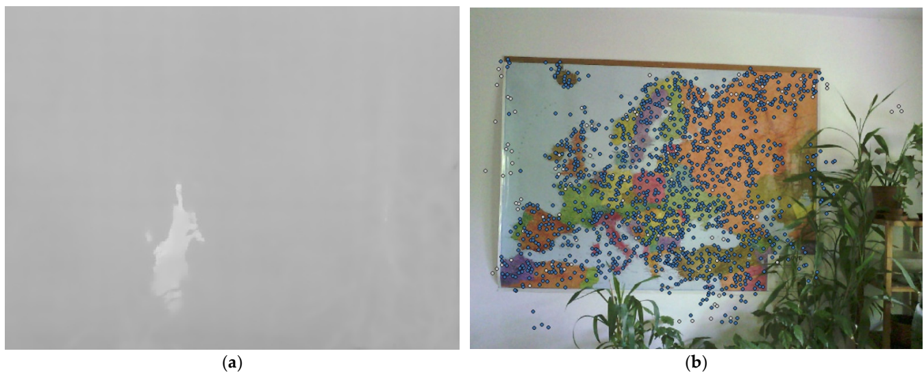
Figure 1. TIR and RGB image of the same scene: (a) feature matching algorithm failed to find any key point or tie point; (b) feature matching algorithm found sufficient amount of tie points (blue dots).
