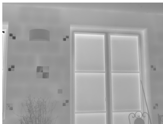
Figure 4. Image captured from 4 m distance. In the image are recognizable cross aluminum paper targets.
